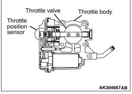
The throttle position sensor, which is built into the throttle body, inputs a voltage that corresponds to the rotational angle of the throttle shaft into the engine-ECU or engine-A-M/T-ECU.
