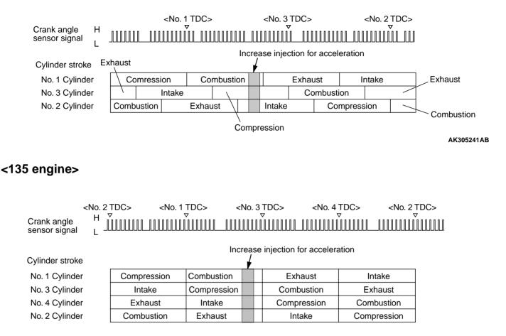
During acceleration, a volume of fuel is injected in accordance with the extent of acceleration, in addition to the fuel that is injected in sync with the crank angle sensor signals.
