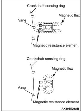
As the sensing ring rotates, the vanes of the sensing ring pass in front of the crank angle sensor (sensing unit).
