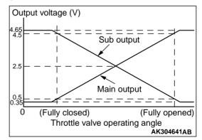
The diagram describes the relationship between the extent of the opening of the throttle and the output voltage.
