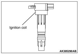
The ignition coils generate high voltage that is required for igniting the spark plugs in accordance with the ignition signals provided by the engine-ECU or engine-A-M/T-ECU.
