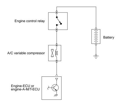
When an A/C variable compressor actuation signal is input by the A/C-ECU via CAN communication, the engine-ECU or engine-A-M/T-ECU turns ON the power transistor for actuating the A/C variable compressor, thus actuating the A/C variable compressor. To prevent vibrations while the A/C variable com-
