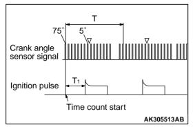
The length of time (t) required for the crankshaft to turn  $1^{\circ}$  is obtained from cycle (T), as follows:
