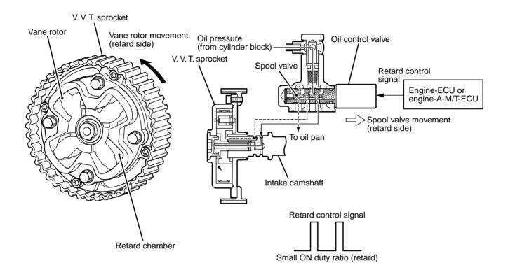
• The spool valve in the oil control valve moves towards timing retard in accordance with the timing advance control signal from the engine-ECU or engine-A-M/T-ECU.
