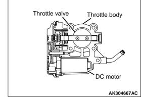
The throttle valve control servo, which is built into the throttle body, opens and closes the throttle valve in accordance with the signals provided by the engine-ECU or engine-A-M/T-ECU. The engine-ECU or engine-A-M/T-ECU determines the extent of the opening of the throttle valve in accordance with the signals provided by the crank angle sensor and the accelerator pedal position sensor, and controls the direction of current applied to the motor and its amperage.
