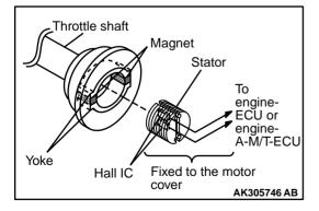
The throttle position sensor consists of a permanent magnet that is mounted on the throttle shaft, a Hall IC that outputs a voltage in accordance with the magnetic flux density, and a stator that effectively guides the magnetic flux from the permanent magnet to the Hall IC.
