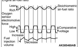
If the actual air-fuel ratio is richer than the stoichiometric air-fuel ratio, the oxygen concentration in the exhaust gases is low. Therefore, the oxygen sensor will input a high electromotive force (rich signal) into the engine-ECU or engine-A-M/T-ECU.
