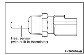
The engine coolant temperature sensor, which is mounted on the cylinder head, detects the temperature of the engine coolant through the changes in the resistance of its thermistor.
