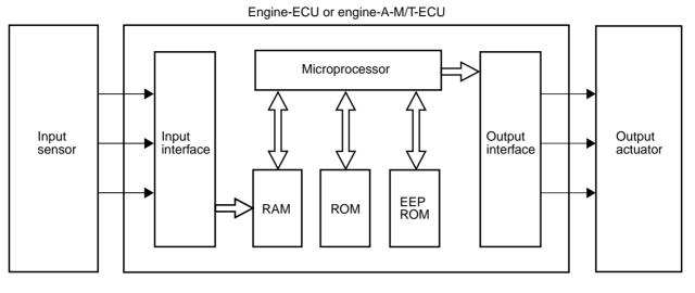
In accordance with the data input by the sensors, the engine-ECU or engine-A-M/T-ECU determines (calculates) optimal control and actuates the output actuators to suit the constantly changing driving conditions.
