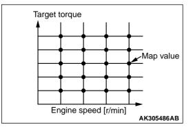
The target phase angle is read by way of the map value that is preset for the respective engine speed and target torque.
