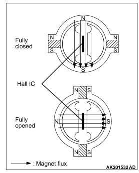
When the throttle valve is fully closed, the density of the magnetic flux that passes through the Hall IC is the lowest.
