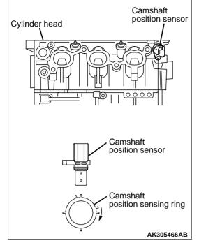
The camshaft position sensor is used for identifying the cylinders jointly with the crank angle sensor. The camshaft position sensor consists of a sensing ring that is mounted on the rear end of the intake camshaft, and a camshaft position sensor (sensing unit) that is mounted on the rear end of the cylinder head.
