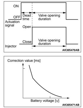
The injector valve opens in accordance with the actuation signals provided by the engine-ECU or engine-A-M/T-ECU. This action is delayed as the battery voltage decreases, making the injector spray a lower volume of fuel than the target fuel injection volume. For this reason, a correction is made in accordance with the battery voltage.
