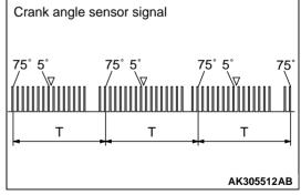
The cycle is measured by using the 75° BTDC signal of the crank angle sensor as a reference. The subsequent cycle is forecast in accordance with the cycle (T) that has been measured currently. The subsequent cycle that has been forecasted will be used for calculating the ignition timing.
