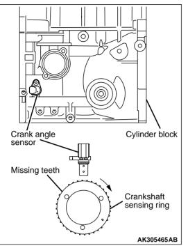
The crank angle sensor detects the crank angle for each cylinder.
