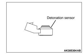
The detonation sensor is mounted at a position in which it can accurately detect the knocking that occurs in the cylinders. It detects the vibration of the cylinder block caused by knocking and outputs a voltage that is proportionate to the extent of the knocking.
