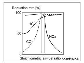
Thus, the system effects feedback control in order to achieve the stoichiometric air-fuel ratio in which the reduction rate of the three-way catalyst is at the optimal level.
