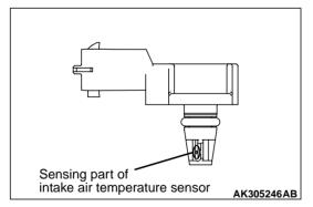
The intake air temperature sensor, which is built into the manifold absolute pressure (MAP) sensor, detects the intake air temperature through the changes in the resistance of its thermistor. The engine-ECU or engine-A-M/T-ECU detects the intake air temperature based on this output voltage and corrects the fuel injection volume to suit the intake air temperature.
