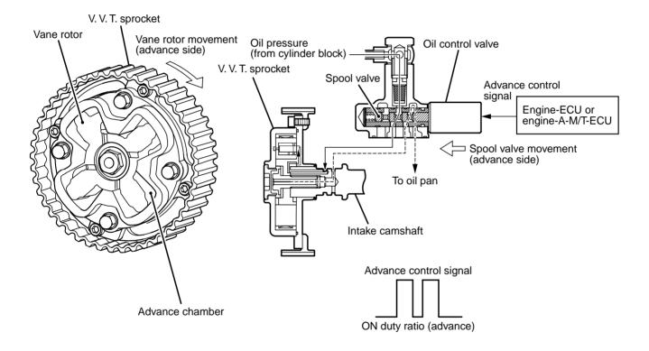
• The spool valve in the oil control valve moves towards timing advance in accordance with the timing advance control signal from the engine-ECU or engine-A-M/T-ECU.
