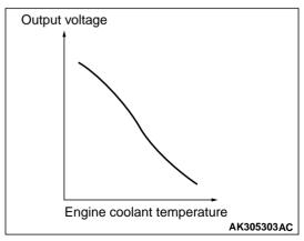
The diagram describes the characteristics of this sensor.
