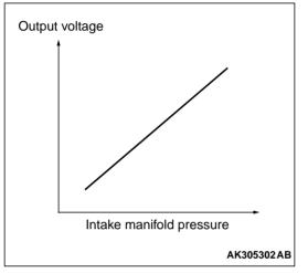
The diagram describes the characteristics of this sensor.
