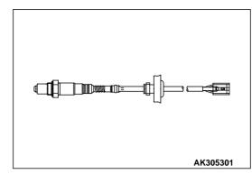
The oxygen sensors are mounted in upstream and downstream of the catalytic converter. Each sensor has a built-in heater for accelerating the activation of the sensor. This feature enables the system to effect air-fuel ratio feedback control in a short time, immediately after the engine has been started.
