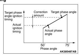
Due to mechanical constraints, the actual phase angle is late in responding to the changes in the target phase angle. Therefore, until the actual phase angle catches up with the target phase angle, the ignition timing is corrected in accordance with the deviation between the target phase angle and the actual phase angle.
