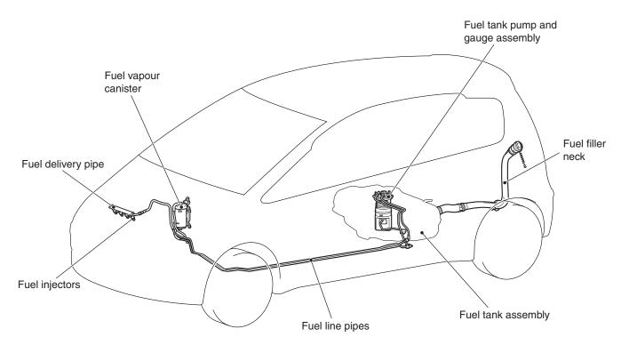
This fuel system is designed with consideration for global environment protection to ensure safety at a collision, reduce weight, and improve reliability and quality. This system has the following features:
