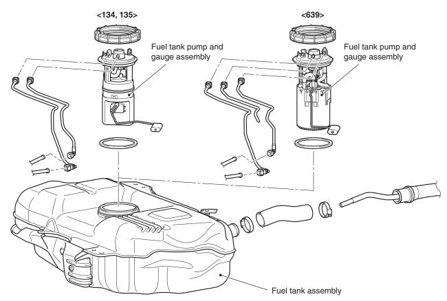
The fuel tank assembly is installed under the rear seat floor, and includes the fuel tank pump and gauge assembly. Its features are as follows:
