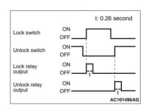
When the driver's door is locked (when the lock switch turns ON after turning OFF the unlock switch in the driver's door lock actuator), ETACS-ECU turns ON the lock relay output for 0.26 second, and locks all doors (including the tailgate). When the driver's door is unlocked (when the unlock switch turns ON after turning OFF the lock switch on the driver's door lock actuator), ETACS-ECU turns ON the unlock relay output for 0.26 second, and unlocks all doors (including the tailgate).
