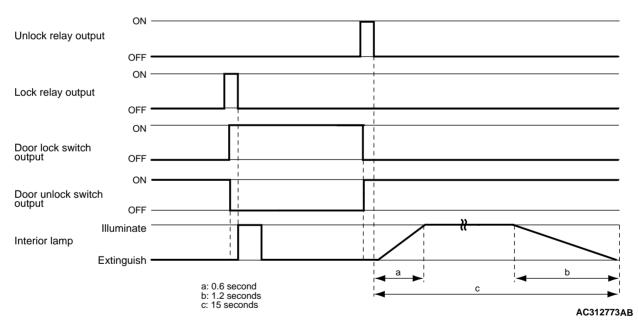
When LOCK signal from the keyless entry transmitter is input to the ETACS-ECU, all doors (including tailgate) are locked and the interior lamp flashes once. When UNLOCK signal is input, all doors (including tailgate) are unlocked and the interior lamp illuminates for 15 seconds. The interior lamp fades in, keeps on, and fades out in 15 seconds after the door unlock relay is operated.
