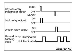
When LOCK signal from the keyless entry transmitter is input to the ETACS-ECU, all doors (including tailgate) are locked and the hazard warning lamp flashes once. When UNLOCK signal is input, all doors (including tailgate) are unlocked and the hazard warning lamp flashes twice.
