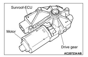
The sunroof motor, which consists of the motor body, drive gear, and sunroof ECU, is installed in front of the housing.
