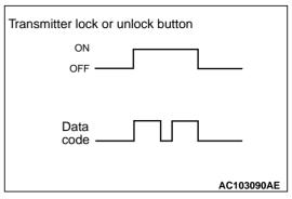
The figure above shows the codes transmitted from the transmitter. Every time the button is pressed, the data code is transmitted twice. The secret code for user identification is a combination of 0 and 1, and more than 1 million different combinations are available. In addition to the secret code, the data code contains a rolling code which changes at each transmission, protecting transmission codes from theft by coping.
