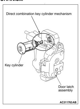
This mechanism allows the doors not to be locked easily during side collision. Because of this, the doors can be opened after side collision.
