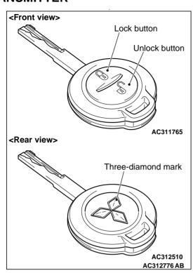
The transmitter is integrated into the master key.
