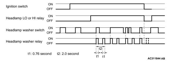
When the headlamp washer switch is turned ON while the ignition switch is in the "ON" position and the headlamp is on (either in Lo-beam or Hi-beam), the headlamp washer control turns ON the headlamp washer relay twice for 0.76 seconds in each cycle.
