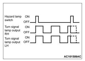
When the hazard lamp switch input signal turning from OFF to ON is detected, the flashing states turns over by the signal (When the hazard lamp is not blinking, it blinks. If it is blinking, it turns off).
