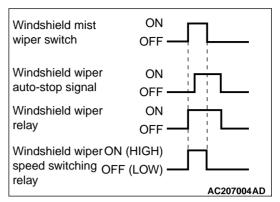
When the windshield mist wiper switch of the column switch is turned ON with the ignition switch in the ACC or ON position, ETACS-ECU turns ON the windshield wiper drive signal. At the same time, the wiper speed switch relay turns to ON (HI). When the windshield mist wiper switch is ON, the windshield wiper operates at the high speed.
