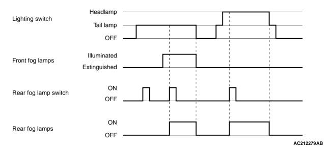
If the rear fog lamp switch is turned ON when the headlamp or the front fog lamp is turned ON, the rear fog lamp is switched ON and OFF alternatively. If the headlamp and the front fog lamp are turned OFF, the rear fog lamp is turned OFF at the same time.
