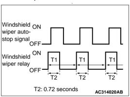
When ETACS-ECU receives the windshield intermittent wiper switch ON signal from the column switch while the ignition switch is in the ACC or ON position, it turns the windshield wiper relay ON to operate the windshield wiper at low speed.
