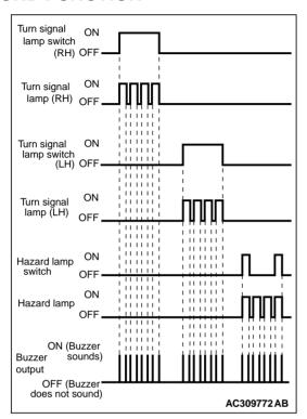
ETACS-ECU buzzer sounds simultaneously with the blinks of the turn signal lamp and the hazard lamp.
