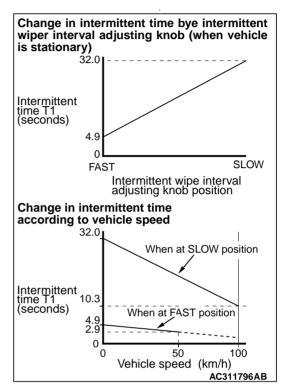
ETACS-ECU calculates the intermittent time T1 based on the variable intermittent wiper volume switch signal sent from the column switch, and on the vehicle speed signal sent from the combination meter through CAN communication.
