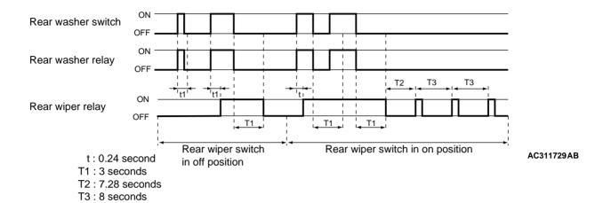
When the rear washer switch on the column switch is turned ON with the ignition switch ACC or ON, ETACS-ECU turns ON the rear washer relay. When the rear washer switch is turned ON for 0.24 second or more, ETACS-ECU will turn ON the rear wiper drive signal and operate the rear wiper continuously. The rear wiper will stop 3 seconds after the rear washer switch has been turned OFF.
