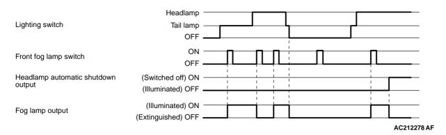
When the fog lamp switch is turned to ON with the tail lamp or the headlamp lit (the tail lamp switch or the headlamp switch is ON), the fog lamp relay turns ON, and the fog lamps turn on.
