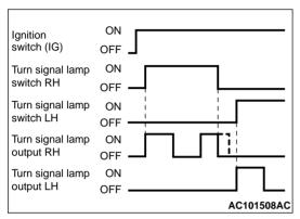
When the turn signal lamp switch is ON (LH or RH) with the ignition switch ON, the turn signal lamp output (flash signal) is turned ON.
