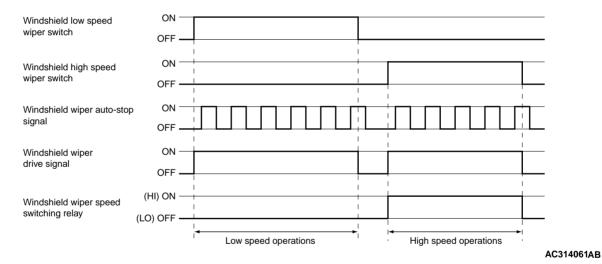
When the windshield low speed wiper switch of the column switch is turned ON while the ignition switch is ACC or ON, the column switch turns ON the windshield wiper drive signal. Also, the wiper speed switching relay turns to OFF (LO), and the windshield wiper operates at the low speed.
