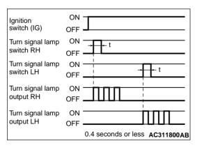
When the turn signal lamp switch is turned ON momentarily (0.4 seconds or less) while the ignition switch is in the "ON" position, the turn signal lamp (selected side) flashes 3 times.
