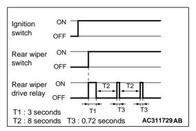
When the rear wiper switch on the column switch is turned ON with the ignition switch at the ACC or ON position, ETACS-ECU turns ON the rear wiper drive signal for 3 seconds (approximately 2 operations), and performs the intermittent action at 8-second intervals
