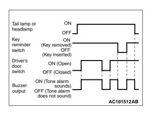
When the ignition key is removed and then the driver's door is opened with turning ON the tail lamp or the head lamp, the buzzer sounds continuously to alert the driver that the lamp is still ON.
