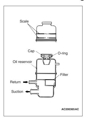
The resin oil reservoir is used to reduce weight. The oil reservoir is translucent and has fluid level marks (MAX and MIN lines), facilitating inspection.
