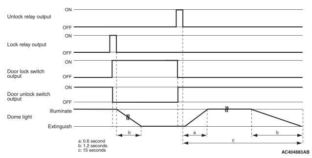
When LOCK signal from the transmitter is input to the ETACS-ECU via WCM, all doors are locked and the dome light will extinguish\*. When UNLOCK signal is input, all doors are unlocked and the dome light illuminates for 15 seconds. The dome light fades in, keeps on, and fades out in 15 seconds after the door unlock relay is operated.
