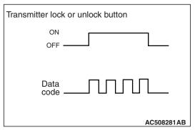
Four data codes are transmitted when a switch is operated once. The encrypted code for user identification is a combination of 0 and 1, and more than 1 million different combinations are available. To prevent theft by copying signal codes, the data code includes a rolling code with the encrypted code. The rolling code changes each time a signal is sent.
