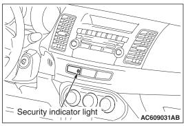
The security indicator light has been installed on the center panel of the instrument panel.
