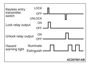
The hazard answerback function that allows checking the lock/unlock state of the door easily even in the daytime is installed. When the LOCK signal from the transmitter is input to ETACS-ECU, all doors are locked and the hazard warning light flashes once. When UNLOCK signal is input, all doors are unlocked and the hazard warning light flashes twice.
