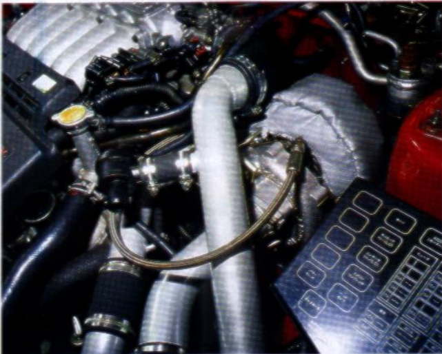
Over the other side of the engine bay, the turbocharger dominates proceedings. Note the location of the turbine blanket
