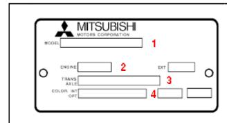
The identification plate is rivetted to the under side of the bonnet.
