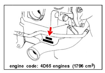
The engine fitted is a 4-cylinder in line engine with overhead camshaft driven by a toothed belt. The injection pump is also driven by this belt.
