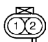
98E12421 Fig. 8: EVAP Purge Solenoid Terminals (Eclipse 2.0L Turbo & 2.4L) Courtesy of Mitsubishi Motor Sales of America
