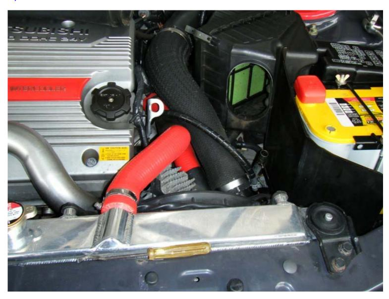
9.) Remove Cold Side Hose to plenum. (NOTE:: you don't need to remove this if your car is not equipped with A/T Filter MD752072)
