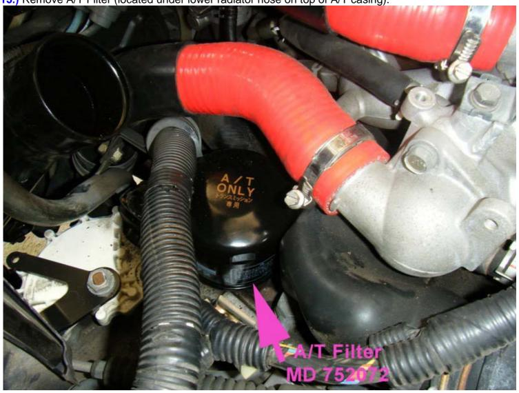
It can be difficult to remove Filter, I've found driving a set of solid tin snips through top of filter and use a Shifter to undo the filter while applying downward force on the tin snip, works best. Making sure that you pierce the filter top allowing maximum usable space for turning the shifter.
