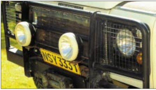
This lightweight bull bar weighs less than 15 kgs, complete with headlight protection and grille net.
