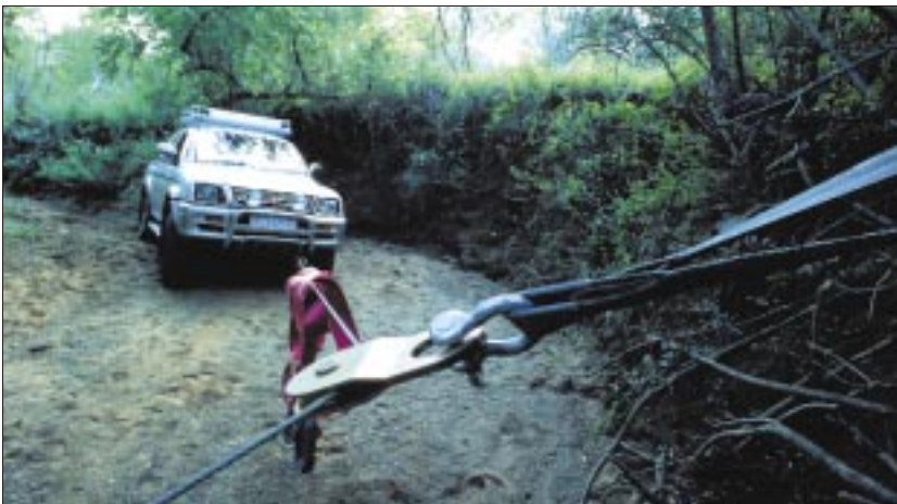
The winch cable is passed through the snatch block and is then returned and attached to a towing eye
