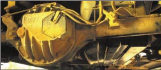
Gearmax differential locks can be fitted to any South African-made rear axle.
