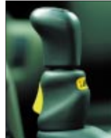
The Freelander's hill-descent control button is found on the gearshift.
