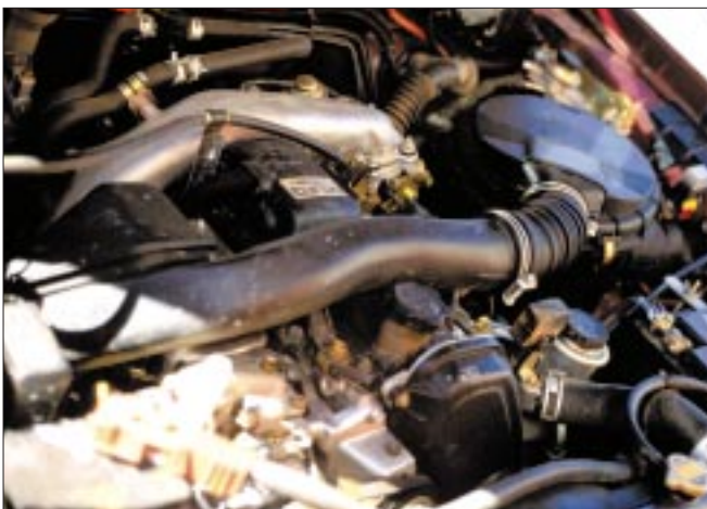
Toyota Land Cruiser Prado 4-cylinder in-line 3-litre turbo-charged diesel is typical of modern turbo-diesel engines. It is superb for off-road use as it produces enough torque before the turbo boosts power to allow easy off-road manoeuvring at very low engine speeds.
