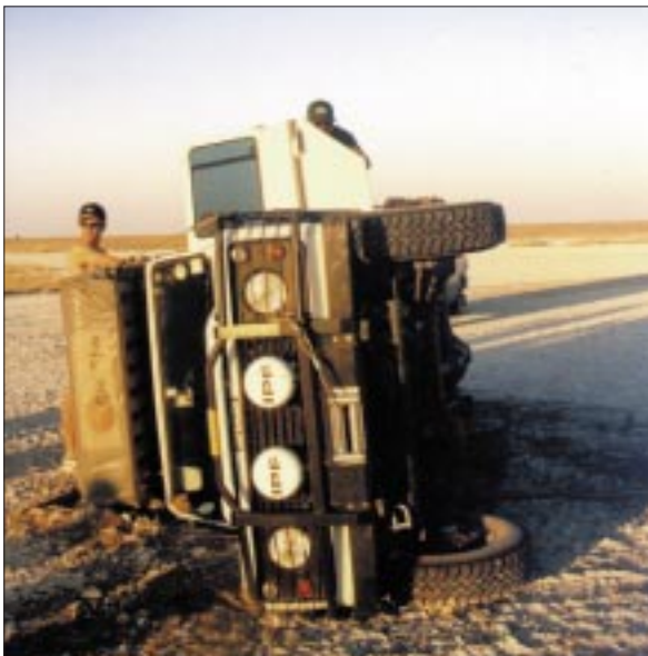
This One Ten rolled during a low-speed pancake on a salt pan. The weight-bearing properties of the crust are often indiscernable from the surface.
