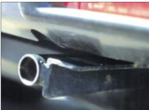
High-lift jack points on a Prado
