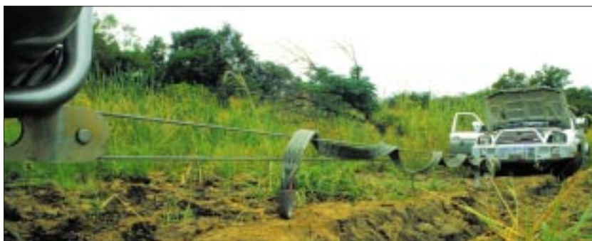
A simple safety line is created by winding a snatch strap over the cable. Should the cable break the extra weight and drag will bring it down quickly and safely.
