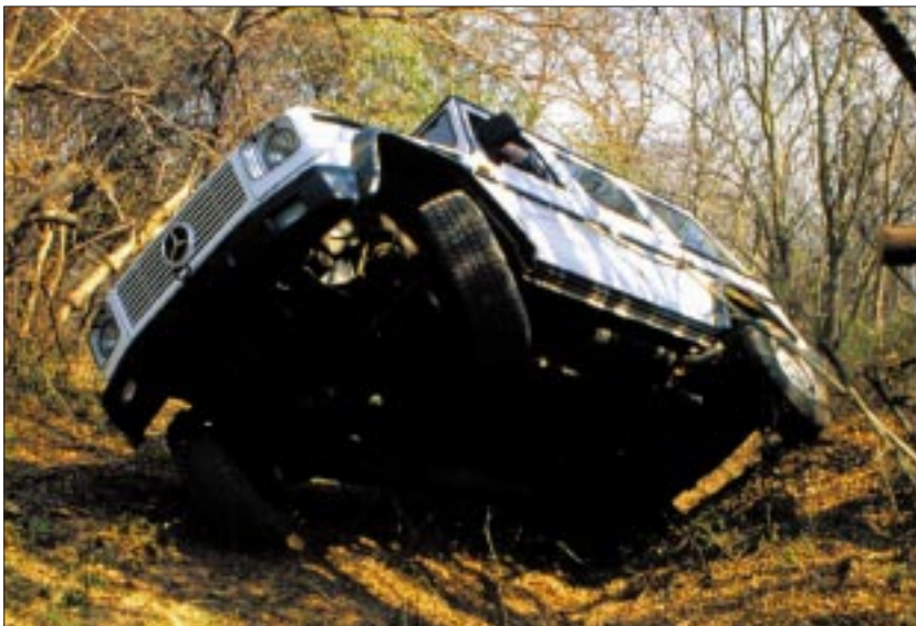
With a low centre of gravity and well-tuned suspension such as the Mercedes G-wagen has, at no time during this axle-twisting obstacle did the vehicle feel as if was going to roll over. If this vehicle had been equipped with a roof-rack I would not have attempted this obstacle. Note the rear wheels firmly on the ground.
