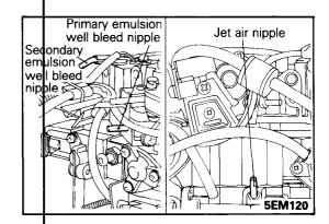
(3) Disconnect the vacuum hoses (black, red stripe, black) from the carburetor primary emulsion well bleed nipple, secondary emulsion well bleed nipple and jet air nipple.
