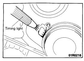
(6) Run the engine at ilde and check ignition timing.
