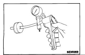
(2) Connect a hand vacuum pump to the check valve and check air tightness.
