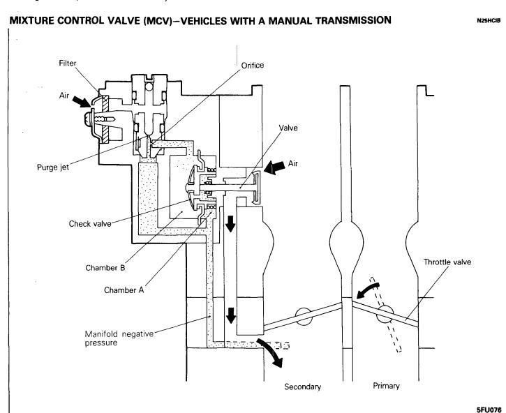
When the throttle is closed suddenly during deceleration or shifting, the fuel remaining in the inlet manifold causes an over rich mixture temporarily.
