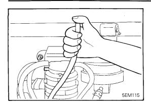
(7) While running the engine at idle, disconnect the vacuum hose (white stripe, two nipples side) from the HAC and hold a finger at the hose end to check that vacuum is felt.
