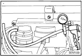
INSPECTION OF HIGH ALTITUDE COMPENSATOR (HAC) — High altitude specifications for the 49 states (excluding California)
