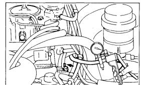
(1) Disconnect the black vacuum hose from the intake manifold nipple and plug the nipple. Then, connect a hand vacuum pump to the disconnected black vacuum hose.
