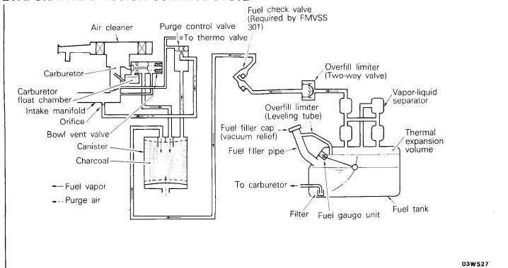
In order to prevent the loss of fuel vapor from the fuel system into the atmosphere, the evaporative emission control system consists of charcoal canister, a bowl vent valve, a purge control valve, etc.
