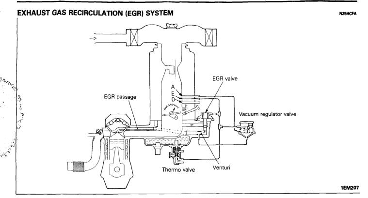
Exhaust Gas Recirculation (EGR) system is designed to reduce oxides of nitrogen in the vehicle exhaust. In this system, the exhaust gas is partially recirculated from an exhaust port at the cylinder head into a port located at the intake manifold while the EGR flow is controlled by an EGR control valve, a vacuum regulator valve (VRV), and a thermo valve.
