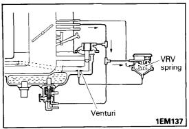
When the venturi pressure drops to near the atmospheric pressure, the VRV opens to allow the E port vacuum to escape to atmosphere. Then, the EGR valve closes.
