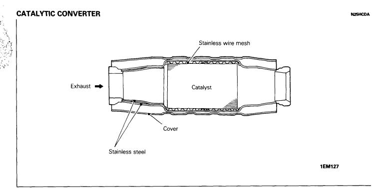
The three catalyst converter which is a monolithic type with catalytic compositions applied to the integrally constructed honeycomb carrier surface is installed in the center of the exhaust pipe. The converter working in combination with the air fuel ratio feedback control oxidizes CO and HC and reduce NOx.
