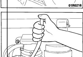
(5) Connect the disconnected vacuum hoses to original position.
