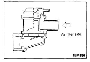
(2) Blow in air from the air filter side to check that air does not blow through.
