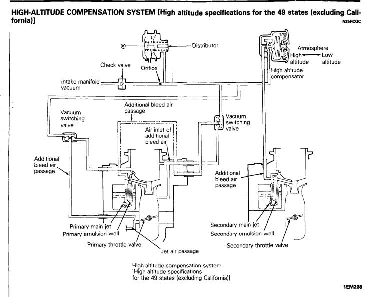
In order to meet the high-altitude requirements for the 49 states (ex. California), all the high-altitude specification carburetor vehicles are equipped with high altitude compensation system in addition to feedback carburetor system.
