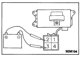
(4) Apply vacuum and check air tighteness both when the battery voltage is applied directly to the solenoid valve terminal and when not applied
