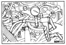
(4) Connect a hand vacuum pump to the vacuum hose and while running the engine at idle, apply vacuum to check the pressure leaks and does not build up.
