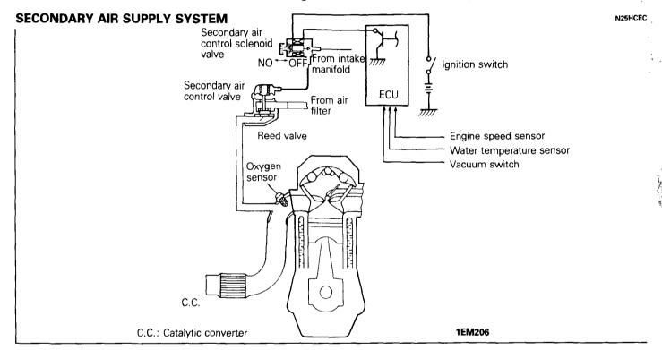
The reed valve supplies secondary air into the exhaust manifold for the purpose of promoting oxidation of exhaust emissions. The reed valve is actuated by exhaust vacuum being generated from pulsation in the exhaust manifold, and additional air is supplied into the exhaust manifold through the secondary air control valve.
