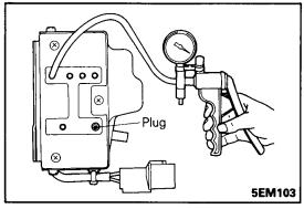
(3) Connect a hand vacuum pump to the nipple to which red stripe vacuum hose has been connected.
