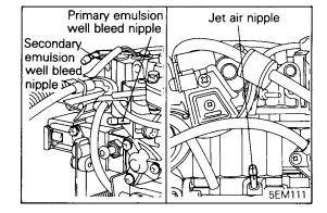
(3) Disconnect the vacuum hoses (black, red stripe, black) from the carburetor primary emulsion well bleed nipple, secondary emulsion well bleed nipple and jet air nipple and plug the nipples.
