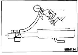
(4) Check air control valve operation.
