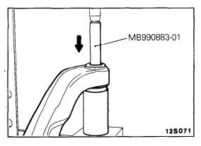
3. Remove the bushing B from the lower arm by using special tools.
