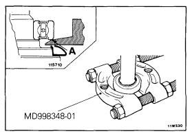
(2) After the special tool has been installed as shown, tighten the nut of the special tool until the portion "A" of the special tool touches the bearing outer race.
