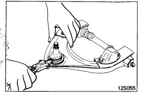
5. Using a snap ring pliers, fit the snap ring securely in the groove of the joint case.
