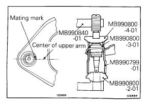
4. Press-fit the new upper ball joint with special tools aligning the mating mark with the upper arm center.
