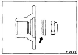
(3) Apply a thin coat of specified grease to the companion flange contacting surface of the washer before installing drive pinion assembly.
