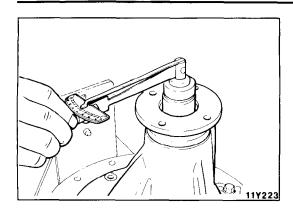
(3) Measure the drive pinion rotation torque (without the oil seal).
