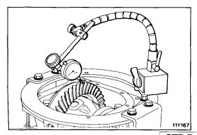
(7) With the drive pinion locked in place, measure the final drive gear backlash with a dial indicator on the drive gear.
