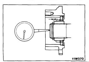
(4) Turn the companion flange counterclockwise until all play is removed and measure the amount of distance through which the mating marks moved.
