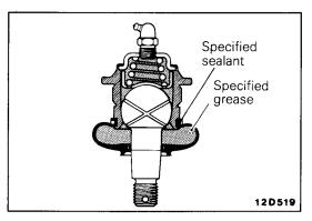
6. Apply the specified grease to both the interior of dust cover and the upper ball joint.
