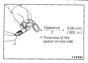
(3) Measure the thickness of the side bearing adjusting spacers on one side, select two pairs of spacers which correspond to that thickness plus one half of the clearance plus 0.05 mm (.002 in.), and then install one pair each to the drive pinion side and the drive gear side.
