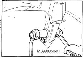
2. Using a special tool, press-fit the bushing A into the bracket.
