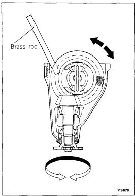
(2) Insert the brass between the differential carrier and the differential case, and then rotate the companion flange by hand (once in the normal direction, and then once in the reverse direction) while applying a load to the drive gear so that the revolution torque [approximately 2.5 to 3.0 Nm (1.8 to 2.2 ft.lbs.)] is applied to the drive pinion.
