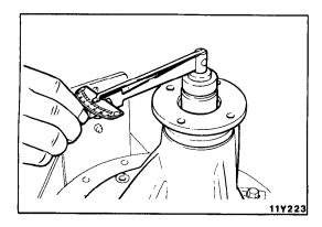
(5) Measure the drive pinion rotation torque (with oil seal) to verify that the drive pinion preload complies with the standard value.
