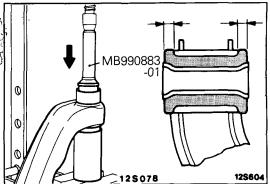
4. Coat the bushing B and the lower arm with soap solution and press-fit the bushing B into the lower arm by using special tools and taking care not to twist or tilt the bushing В.
