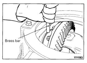
(5) Tap the side bearing adjusting spacers with the brass bar to fit them to the side bearing outer race.
