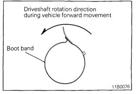
(4) Secure the B.J. boot to the driveshaft by boot bands A and B.
