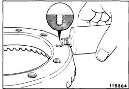
(3) Apply the specified adhesive to the threaded holes of the drive gear.
