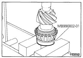
(4) Position the special tool in the side bearing seat of the gear carrier, and then select a drive pinion front shim of a thickness which corresponds to the gap between the special tools.
