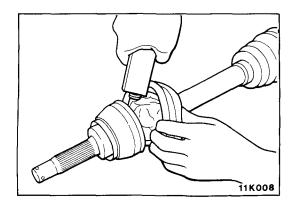
(3) Apply all the specified grease, half of it to the inner side of the B.J., and the other half to the inner side of the B.J. boot.
