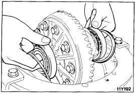
(4)Install the side bearing adjusting spacers and differential case assembly, as shown in the illustration, to the gear carrier.
