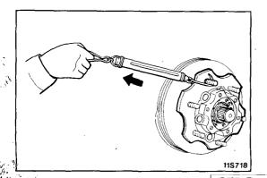
(2) Loosen the lock nut approximately 30 to 40 degrees to adjust the front hub's turning resistance and play in the axial direction so that they agree with the standard values.
