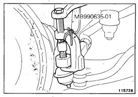
4. DISCONNECTION OF TIE ROD ASSEMBLY FROM KNUCKLE
