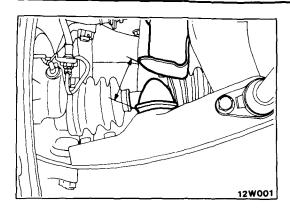
(2) With the vehicle unladen, measure the dimension from the bump stopper to the bump stopper bracket to check for conformance with standard value.
