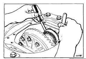
(2) Push the differential case assembly to one side, and measure the clearance between the gear carrier and the side bearing adjusting spacer with a feeler gauge.
