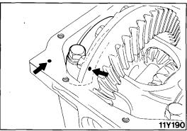
(6) Align the mating marks on the gear carrier and the bearing cap, and then tighten the bearing cap.
