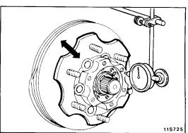
(2) Loosen the lock nut approximately 30 to 40 degrees to adjust the front hub's turning resistance and play in the axial direction so that they agree with the standard values.
