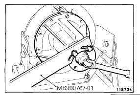
(4) Install the drive pinion assembly and companion flange with mating marks properly aligned, and tighten the companion flange self-locking nut to the specified torque by using the special tools.
