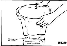
(25)Install the O-ring at illustrated position and then install the converter housing.
