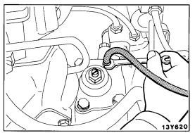
8. Loosen the breather plug, and then turn the steering wheel completely to the right and left continuously until air bubbles no longer appear in the fluid coming out of the tube.
