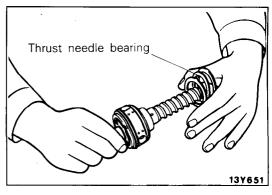
(3) Install the thinner thrust plate, thrust needle bearing and thicker thrust plate to the mainshaft in that order as shown in the illustration.
