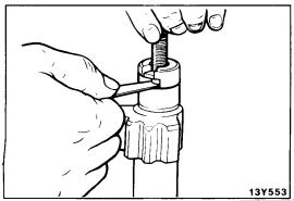
(3) If the end play exceeds the standard value, select a suitable adjusting plate from the table, install it, and then measure the end play once again.
