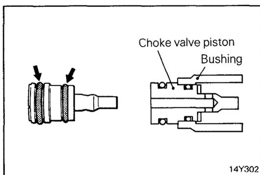
**13. INSTALLATION OF VALVE CAP**
