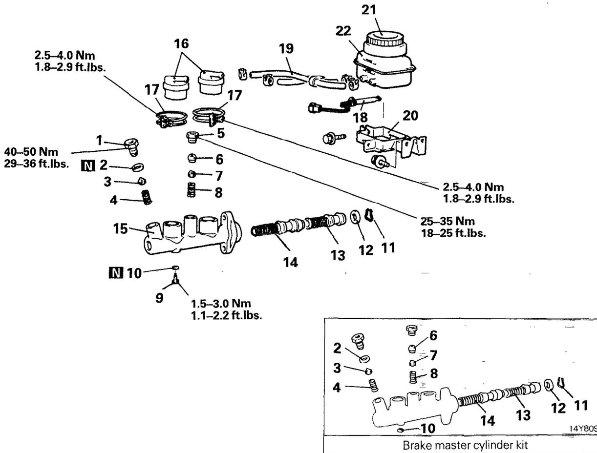
**Brake master cylinder disassembly steps**
