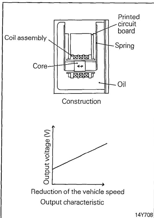
**G-Sensor (Detection of the Reduction of the Vehicle Speed)**
