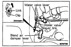
Unfasten the clip of the blend air damper lever, and disconnect the link for water valve lever from the blend air damper lever.
