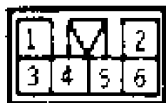
Fig. 11: Vacuum Pump Connector Terminal ID Courtesy of Mitsubishi Motor Sales of America.
