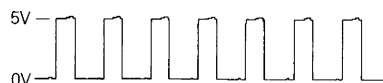
Fig. 25: Known-Good CKP Sensor Wave Pattern ID Courtesy of Mitsubishi Motor Sales of America
