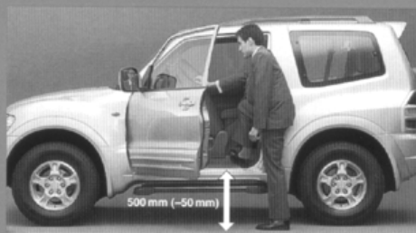
Despite higher ground clearance, the floor height is lower for easier access.
