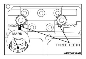
>>U<< SHIFT RAIL DRIVE GEAR INSTALLATION
