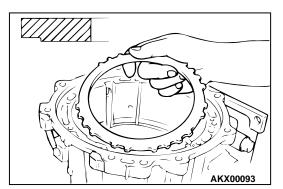
A CAUTION Make sure the reaction plate in the proper direction. 39.Install the reaction plate.
