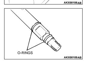
58.Install two new O-rings to the manual control shaft, and assemble onto the transmission case together with the detent lever and parking roller rod.
