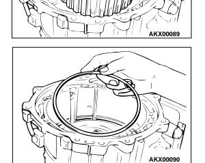
36.Install the wave spring to the low/reverse brake piston.
