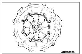
15.Remove the eight converter housing mounting bolts, and then the converter housing.
