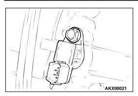
80.Install the input shaft speed sensor.
