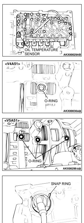
9. Remove the twenty valve body mounting bolts and then remove the valve body, O-ring and oil temperature sensor.
