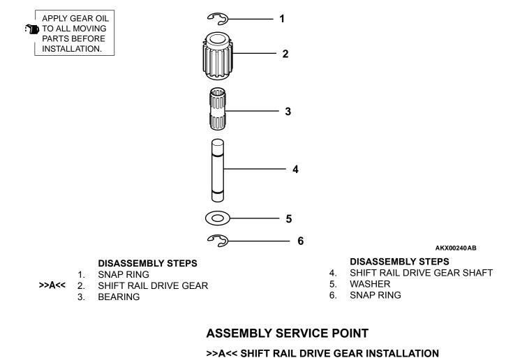
Install so that the mating mark of the shift rail drive gear is opposite side of the washer.
