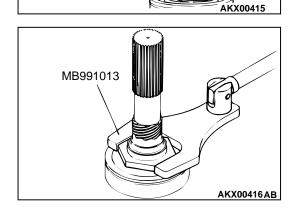
4. Use special tool MB991013 to remove the jam nut.
