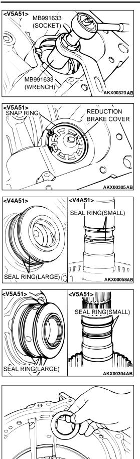
(4) Tighten the reduction brake piston nut to the specified torque using the special tool (wrench) with the special tool (Socket) so it does not rotate.
