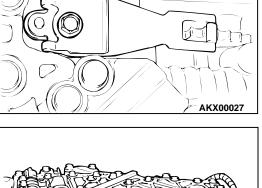
8. Disconnect the valve body harness connectors.
