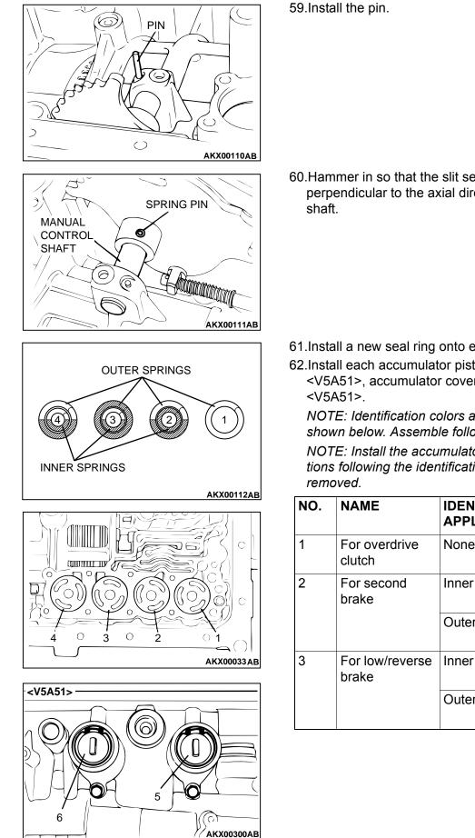
60.Hammer in so that the slit section of the spring valve is perpendicular to the axial direction of the manual control
