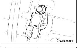
2. Remove the output shaft speed sensor.
