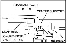
(3) Select the snap ring for fixing the center support installed in step 31 (1) so that the end play of the center support is at the standard value. Then, reassemble.
