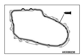
**CAUTION** Squeeze the sealant out evenly to apply it in an unbroken, non-excessive quantity.
