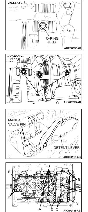
65.Install the new O-ring into the transmission case at the position shown in the illustration.
