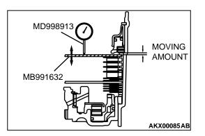
(9) Install a dial gauge onto special tool MD998913 so the end contacts the special tool. Move special tool MB991632 and measure the moving amount. Select a pressure plate with a thickness that corresponds to the measured moving amount from the following table.
