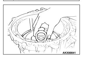
22.Remove the thrust bearing number 4.
