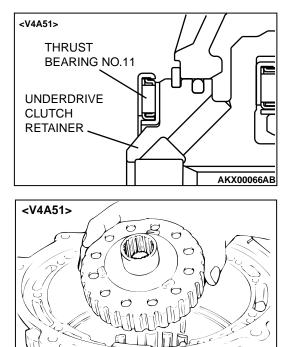
**CAUTION** Make sure thrust bearing number 11 is mounted in the correct direction.
