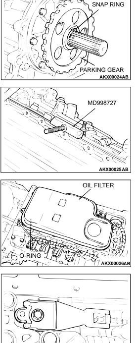
4. Remove the snap ring, and remove the parking gear using a puller [corresponding load approximately 9,800 N (2,200 pounds)].
