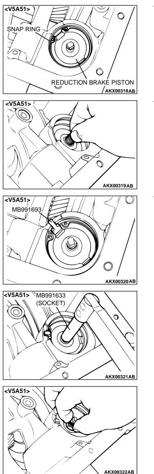
11.Press the reduction brake piston into the transmission case, and then install the snap ring. <V5A51>
