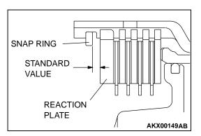
3. Confirm that the clearance (underdrive clutch end play) between the snap ring and reaction plate is the standard value. If the clearance is not at the standard value, select the snap ring and adjust so that the clearance is within the standard value.
