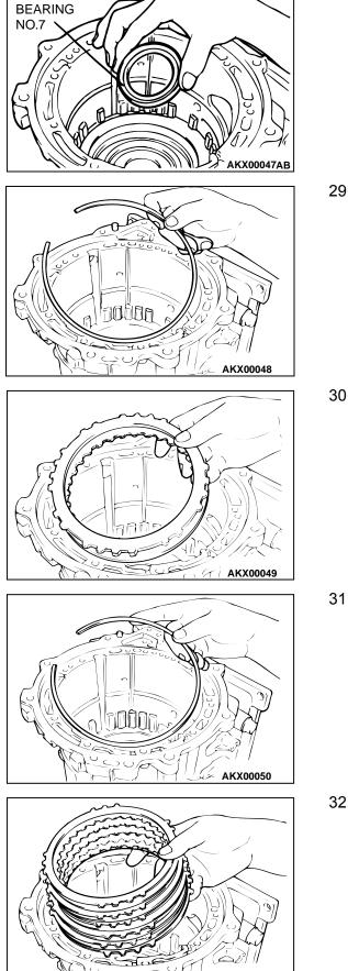
28.Remove the thrust bearing number 7.
