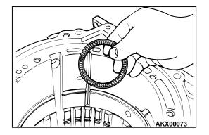
24.Apply Vaseline or petroleum jelly on the thrust bearing number 9, and then install on the output flange <V4A51> or direct annulus gear <V5A51>.
