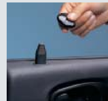
KEYLESS ENTRY A transmitter key activates your central door locking and interior lighting. MZ311929
