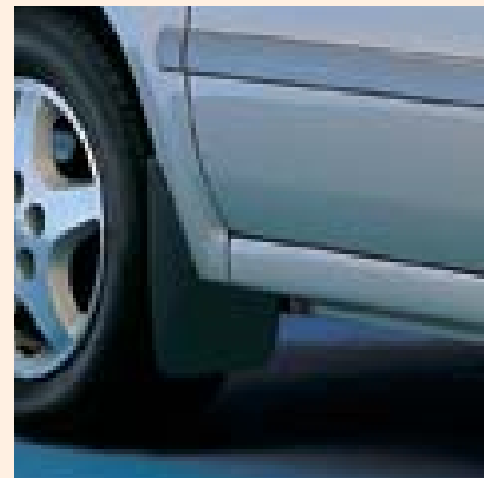
MUDGUARDS FRONT SET For vehicles without side airdam MZ311911 For vehicles with side airdam MZ312250
