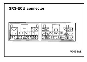
5. Do not attempt to repair the wiring harness connectors of the SRS. If any of the connectors are diagnosed as faulty, replace the wiring harness. If the wires are diagnosed as faulty, replace or repair the wiring harness according to the following table.
