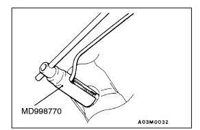
REMOVAL SERVICE POINT AD OXYGEN SENSOR REMOVAL INSTALLATION SERVICE POINT DA OXYGEN SENSOR INSTALLATION 15100540355
