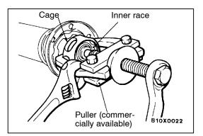
Make mating marks on the outer race, cage and on the inner race, and then remove the outer race and balls. NOTE
