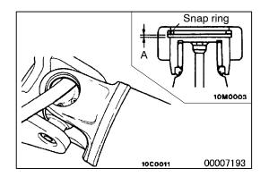
2. Install another snap ring to the opposite snap ring groove, and use a thickness gauge to measure the clearance in the snap ring groove.
