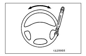
Measure the play on steering wheel circumference before wheels start to move when slightly moving steering wheel in both directions.
