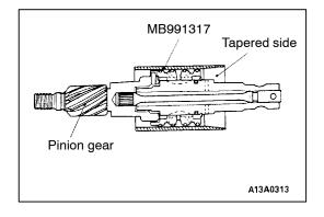
2. Apply the specified fluid to the oil seal inner surface and the O-ring.
