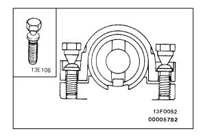
2. After checking that the lock works properly, tighten the special bolts until the head twists off.
