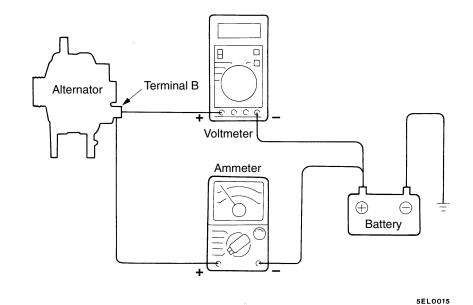
This test determines whether the wiring from the alternator "B" terminal to the battery (+) terminal (including the fusible line) is in a good condition or not.
