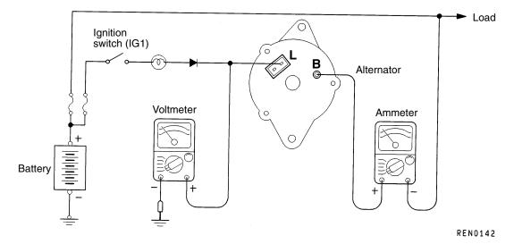
This test determines whether the voltage regulator is correctly controlling the alternator output voltage. (1) Always be sure to check the following before
