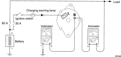
This test determines whether the alternator output current is normal.
