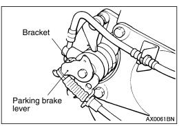
5. After adjusting the parking brake lever stroke, jack up the rear of the vehicle. Release the parking brake and turn the rear wheels to check that the rear brakes are not dragging. In addition, check that the parking brake lever on the caliper side is touching the bracket.
