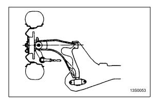
Also the lower arm front bushing is installed at a point almost on the same line as the front wheel axis line to provide increased lateral rigidity and reduced lateral force steering.
