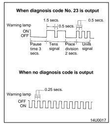
2. Turn the ignition switch to ON and then take a reading of th diagnosis codes from the flashing of the ABS warning lamp.
