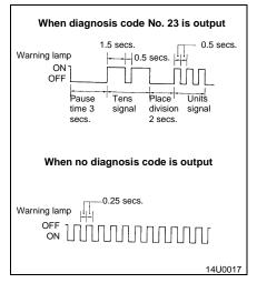
3. Turn the ignition switch to ON and then take a reading of th diagnosis codes from the flashing of the ABS warning lamp.
