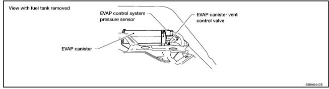
Check sensor harness connector for water.
