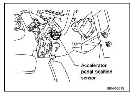
3. Check voltage between APP sensor terminal 7 and ground with CONSULT-II or tester.
