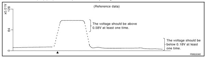
"HO2S2 (B1)/(B2)" should be above 0.58V at least once when the "FUEL INJECTION" is +25%. "HO2S2 (B1)/(B2)" should be below 0.18V at least once when the "FUEL INJECTION" is -25%.
