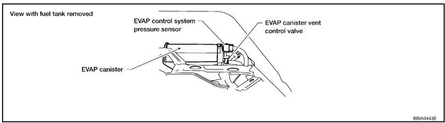
Pressurize the EVAP line using pressure pump with 1.3 to 2.7 kPa (10 to 20 mmHg, 0.39 to 0.79 inHg), then remove pump and EVAP service port adapter.
