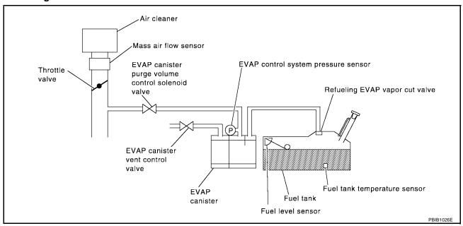
In this evaporative emission (EVAP) control system, purge flow occurs during non-closed throttle conditions. Purge volume is related to air intake volume. Under normal purge conditions (non-closed throttle), the EVAP canister purge volume control solenoid valve is open to admit purge flow. Purge flow exposes the EVAP control system pressure sensor to intake manifold vacuum.
