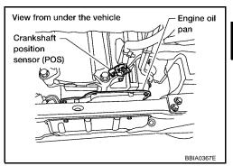
Check voltage between CKP sensor (POS) terminal 3 and ground with CONSULT-II or tester.
