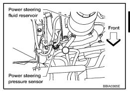
3. Check voltage between PSP sensor terminal 1 and ground with CONSULT-II or tester.
