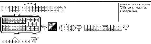
\*: THIS CONNECTOR IS NOT SHOWN IN "HARNESS LAYOUT" OF PG SECTION.
