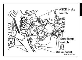
4. Check voltage between ASCD brake switch terminal 1 and ground with CONSULT-II or tester.
