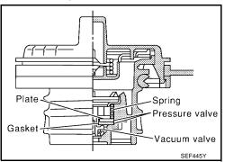
2. Check valve opening pressure and vacuum.
