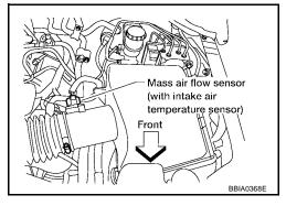
Check voltage between mass air flow sensor terminal 5 and ground.
