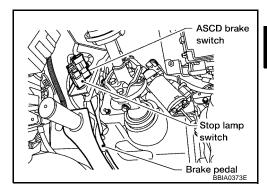
2. Check continuity between stop lamp switch terminals 1 and 2 under the following conditions.
