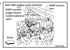
Check voltage between EVAP canister purge volume control solenoid valve terminal 1 and ground with CONSULT-II or tester.
