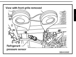
Check voltage between refrigerant pressure sensor terminal 1 and ground with CONSULT-II or tester.
