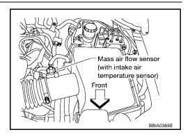
3. Check voltage between MAF sensor terminal 2 and ground with CONSULT-II or tester.
