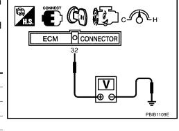
Verify that EVAP control system pressure sensor value stays 0.1V less than the value at idle speed (measured at step 6) for at least 1 second.
