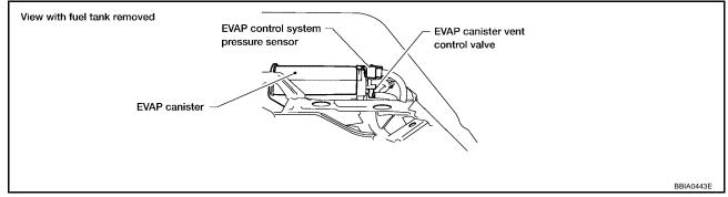
Check sensor harness connector for water.
