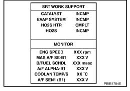
11. Rev engine up to 2,000 to 3,000 rpm and maintain it until "INCMP" of "CATALYST" changes to "CMPLT" (It will take approximately 5 minutes).
