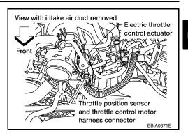
Check voltage between electric throttle control actuator terminal 2 and ground with CONSULT-II or tester.
