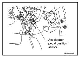
Check voltage between APP sensor terminal 6 and ground with CONSULT-II or tester.
