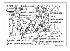
2. Connect ignition coil No.1 and spark plug with suitable high-tension wire as shown, and attach timing light clamp to this wire.
