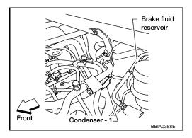
Check voltage between condenser terminal 1 and ground with CONSULT-II or tester.
