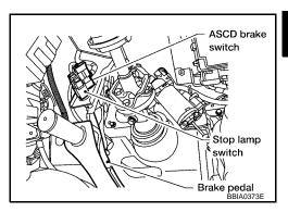
3. Check voltage between stop lamp switch terminal 1 and ground with CONSULT -II or tester.
