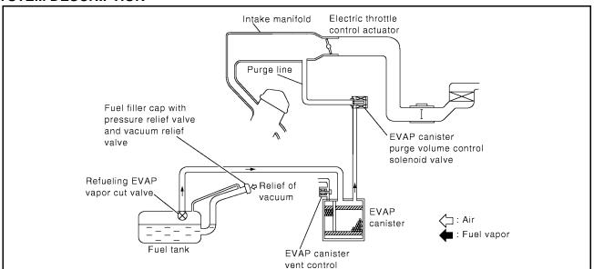
The evaporative emission system is used to reduce hydrocarbons emitted into the atmosphere from the fuel system. This reduction of hydrocarbons is accomplished by activated charcoals in the EVAP canister.
