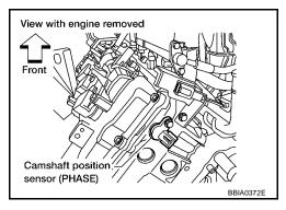
Check voltage between CMP sensor (PHASE) terminal 3 and ground with CONSULT-II or tester.
