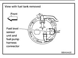
3. Check voltage between "fuel level sensor unit and fuel pump" terminal 4 and ground with CONSULT-II or tester.
