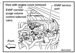
Also attach the pressure pump with pressure gauge to the EVAP service port adapter.
