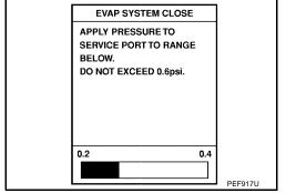
Using EVAP leak detector, locate the EVAP leak. For the leak detector, refer to the instruction manual for more details. Refer to EC-33, "EVAPORATIVE EMISSION LINE DRAWING".
