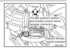
Check voltage between electric throttle control actuator terminal 2 and ground with CONSULT-II or tester.
