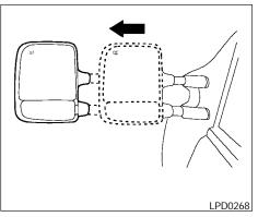
Pull the trailer tow mirror outward to extend it to the desired position for better visibility while towing a trailer.
