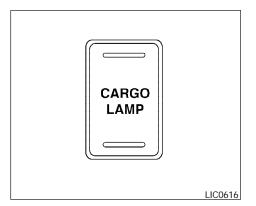
To turn on the cargo lamp, push the switch down to the ON position. The tailgate lights (if so equipped) will also illuminate when the cargo lamp switch is in the ON position.
