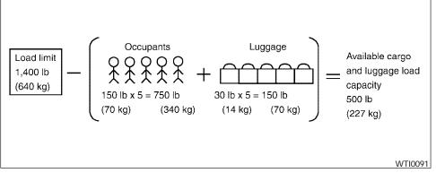
Steps for determining correct load limit
