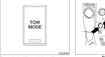
Tow mode should be used when pulling a heavy trailer or hauling a heavy load. Using tow mode at other times may cause unnecessary transmission shifting and reduced fuel economy.
