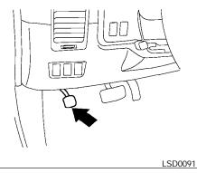
To engage: Firmly depress the parking brake.
