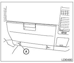
Remove the 2 lower glove box hinge pins
