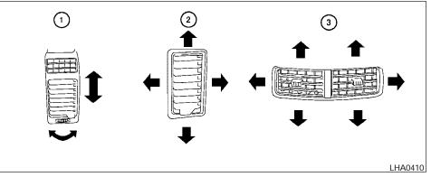
Adjust air flow direction for the driver and passenger side ①, center ②, and rear passenger (if so equipped) ③ ventilators by moving the ventilator slide and/or ventilator assemblies.
