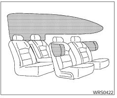
Supplemental side-impact air bag and curtain side-impact and rollover air bags system (if so equipped)
