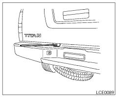
3. Assemble the two pieces of the jack rod. Find the oval-shaped opening above the middle of the license plate. Pass the T-shaped end of the jack rod through the opening and direct it toward the spare tire winch, located directly above the spare tire.
