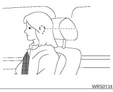
Adjust the head restraint so the center is level with the center of your ears.
