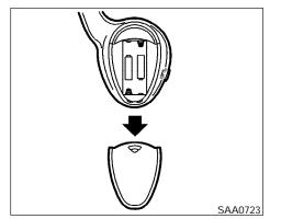
If the battery is removed for any reason other than replacement close the lid securely.
