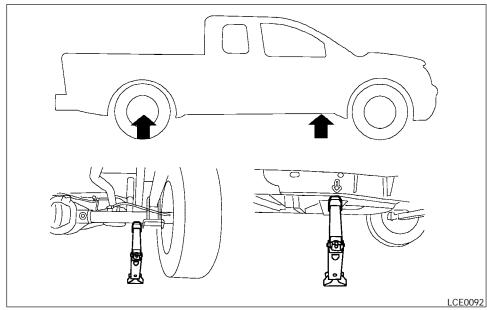
2. Place the jack directly under the jack-up point as illustrated so the top of the jack contacts the vehicle at the jack-up point. The jack-up points are indicated by stamped arrows on the side of the frame. The jack should be used on firm and level ground.
