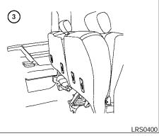
(3) Repeat this process to raise and secure the seat cushion on the other side of the vehicle for maximum storage capacity.
