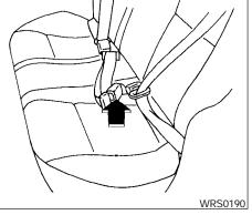
TWO-POINT TYPE SEAT BELT WITHOUT RETRACTOR (center of the front bench seat) (if so equipped)
