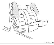
Supplemental side-impact air bag system (if so equipped)
