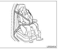
BOOSTER SEAT INSTALLATION ON FRONT PASSENGER SEAT
