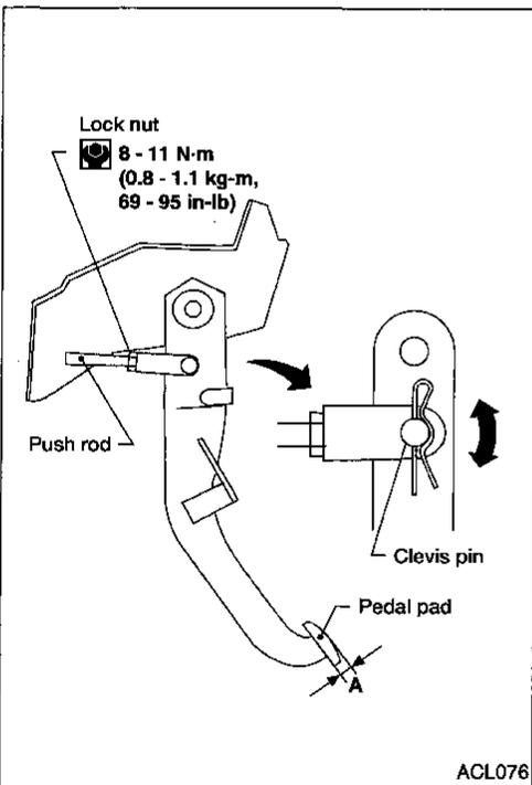
2. Adjust pedal free play by turning master cylinder push rod. Then tighten lock nut.
