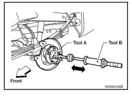
6. Using a puller remove the bearing cup from the rear axle case.
