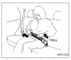
2. Tighten the belt by pulling the free end of the belt away from the tongue.
