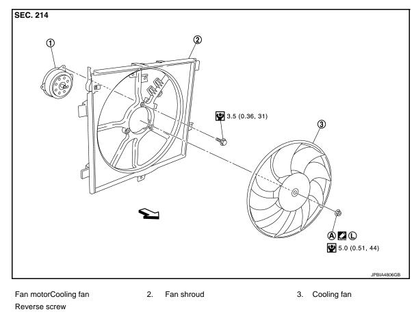
Apply thread locking sealant.
