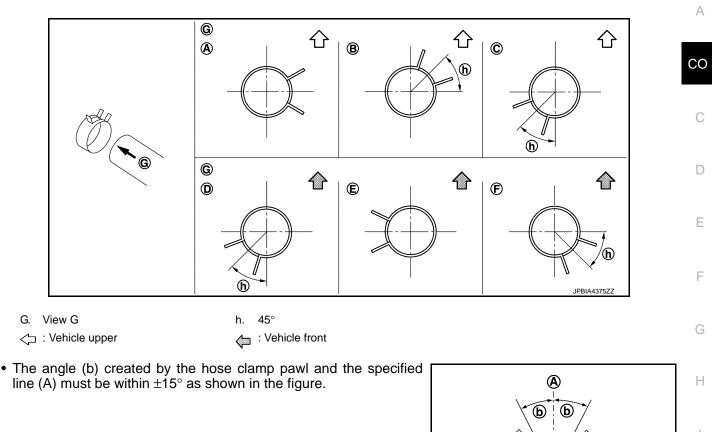
• To install hose clamps (1), check that the dimension (A) from the end of the paint mark (2) on the radiator hose to the hose clamp is within the reference value.
