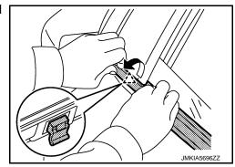
3. Slide rear door outside molding (1) toward vehicle front, and then pull molding out from rear door handle (2).
