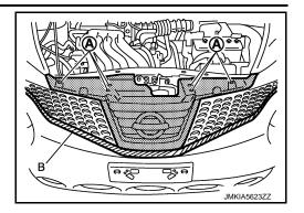
Disengage fixing pawls from back side while pulling front center grille to wade vehicle front, and then remove front center grille.
