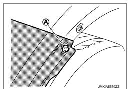
5. Remove air guide fixing screws, and then remove air guide (LH and RH).Refer to <a href="EXT-22">EXT-22</a>. "Exploded View".
