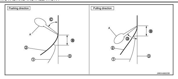
3. For small radius portion of hemming part, gradually apply pressure and affix door sash tape (1) using squeegee (A) in 1-3 steps.
