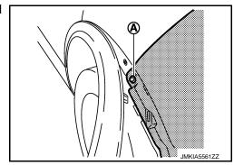
7. Pull bumper fascia side toward the vehicle side to disengage the fitting of bumper side bracket and bumper fascia side as shown by the arrow in the figure.
