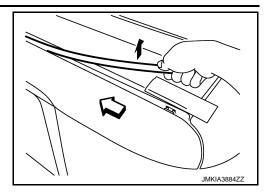
Disengage windshield molding and clip at the front end of roof side molding, and then remove while pulling out toward vehicle rear.
