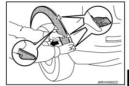
Using remover tool (A), disengage the clips from rear fillet molding by starting from rear side.
