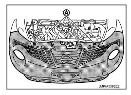
Remove front fillet molding front side. Refer to EXT-26, "FRONT FILLET MOLDING: Removal and Installation".
