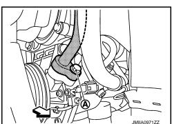
9. Remove low-pressure flexible hose from vehicle.
