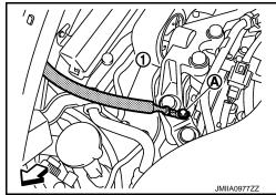
8. Remove mounting bolt (A), and then disconnect low-pressure flexible hose from compressor. **CAUTION:**
