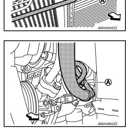
5. Remove high-pressure flexible hose from vehicle.
