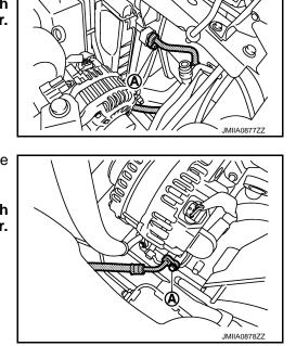
4. Remove high-pressure flexible hose from vehicle.
