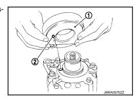
3. Install pulley assembly pulley installer (1) using (SST:KV99106200) (A) and a hand press, and then install snap ring (2) using snap ring pliers.
