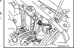
Remove mounting bolt (A), and then disconnect high-pressure pipe from condenser.
