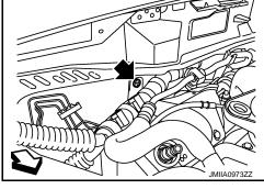
Remove mounting bolt (A), and then disconnect low-pressure flexible hose (1) and high-pressure pipe (2) from expansion valve. Refer to <u>HA-116</u>, "<u>EXPANSION VALVE</u> : <u>Removal and</u> <u>Installation</u>". CAUTION:
