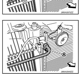
7. Remove mounting bolts, and then remove condenser from the vehicle. CAUTION:
