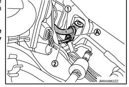
4. Remove mounting bolts (A), and then remove expansion valve from evaporator.
