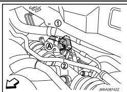
6. Remove mounting bolt (A) of low-pressure flexible hose front side (1) and mounting nut (B) of low-pressure flexible hose rear side (2).
