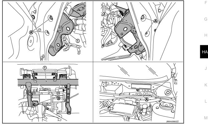
18. Remove A/C unit assembly from vehicle.
