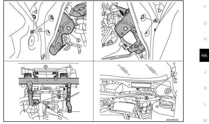
19. Remove A/C unit assembly from vehicle.
