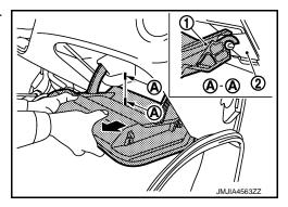
3. Disengage the pawl, and then remove damper pin on right side.
