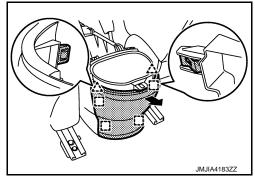
Remove center console assembly fixing screws (A).
