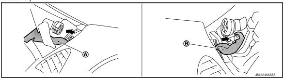
2. Remove instrument panel from passenger door opening portion.
