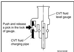
Pull out the CVT fluid level gauge from the CVT fluid charging pipe after pressing the tab on the CVT fluid level gauge to release the lock.
