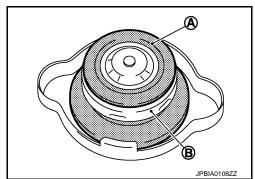
Pull negative-pressure valve to open it, and check that it close completely when released.
