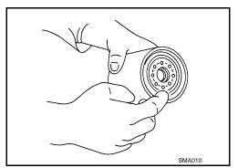
Screw oil filter manually until it touches the installation surface, then tighten it by 2/3 turn (A). Or tighten to specification.
