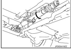
Propeller shaft runout measuring point (Point "△")
