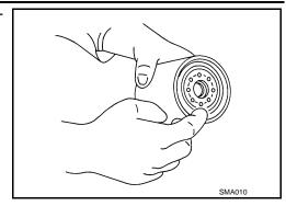
3. Screw oil filter manually until it touches the installation surface, then tighten it by 2/3 turn (A). Or tighten to specification.
