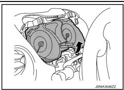
Remove connector to remove the combination meter. CAUTION: Never damage the front cover.
