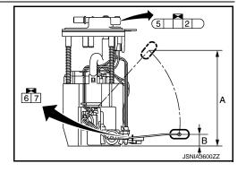
\*: When float rod is contact with stopper.
