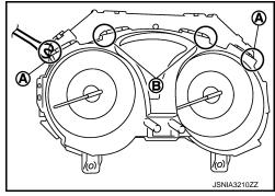
Pull the front cover straight to remove it from the meter control unit assembly. CAUTION: Never damage the front cover.
