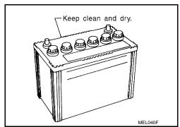
When the vehicle is not going to be used over a long period of time, disconnect the battery cable from the negative terminal. (If the vehicle has an extended storage switch, turn it off.)
