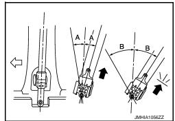
3. Replace the seat belt assembly if it does not operate normally. SEAT BELT BUCKLE
