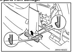
5. Pull up floor carpet and disconnect lap pre-tensioner seat belt harness connector. CAUTION:
