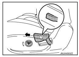
4. Tilt seat toward seat front until fixing screw (A) of seat cushion outer finisher (1) and reclining device outer cover (2) are visible. Remove fixing screw.
