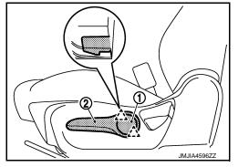
3. Disengage pawl using a screwdriver while pulling reclining lever knob. Slide reclining lever knob toward seat front and remove it.
