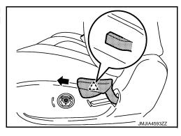
4. Pull seat cushion outer finisher toward seat front. Disengage pawls and metal clips. Slide seat cushion outer finisher toward seat front. Remove seat cushion outer finisher.
