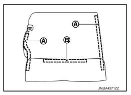
4. Slide and align the clips (B) to the holes on the seatback as shown in the figure, and then remove the seatback board (A).
