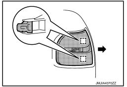
2. Pull tether cover in direction indicated by the arrow as shown in the figure. Remove tether cover.
