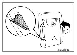
3. Open seatback fastener (A) and remove seatback retainer (B).
