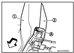
5. Pull seat cushion outer finisher toward seat front. Disengage pawls and clips. Slide seat cushion outer finisher toward seat front. Remove seat cushion outer finisher.
