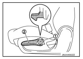
Disengage pawl using a screwdriver while pulling reclining lever knob. Slide reclining lever knob toward seat front and remove it.
