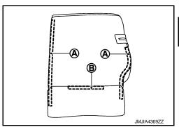
Use pincers, etc., to press up pawls as shown by the arrows in the figure, and remove headrest holder from seatback. CAUTION:
