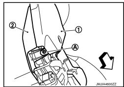
Remove fixing screws. Pull seat cushion inner finisher toward seat front. Disengage pawls. Remove seat cushion inner finisher.
