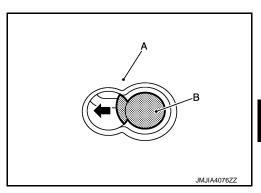
5. Use pincers, etc., to press up pawls as shown by the arrows in the figure, and remove headrest holder from seatback.
