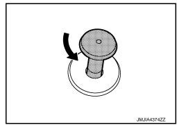
2. Push up seatback lock knob finisher while pressing pawls indicated by arrows as shown in the figure. Remove seatback lock finisher from seatback.
