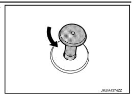
Push up seatback lock knob finisher while pressing pawls indicated by arrows as shown in the figure. Remove seatback lock finisher from seatback.
