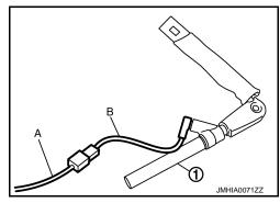
3. Put the lap pre-tensioner (1) connected with the deployment tool into a tire without a wheel.
