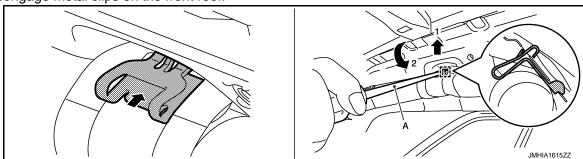
1. Fully insert a flat-bladed screwdriver (A) into center of metal clip.
