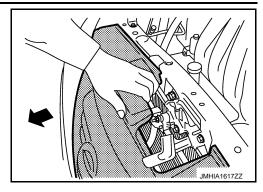
3. Remove the crash zone sensor fixing nuts (A), and then pull the bracket (1) and crash zone sensor (2) for vehicle front.
