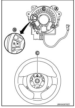
• Fix the driver air bag module harnesses to the harness fixing hook (A).
