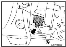
Disconnect the harness connector and then remove the side air bag (satellite) sensor.
