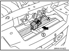
4. Disconnect the crash zone sensor harness connector, and then remove crash zone sensor.
