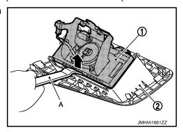
2. Make 8.5 mm (0.335 in) diameter hole (B) in air bag module bracket (SST: KV99105300) (A) at the position shown in figure.
