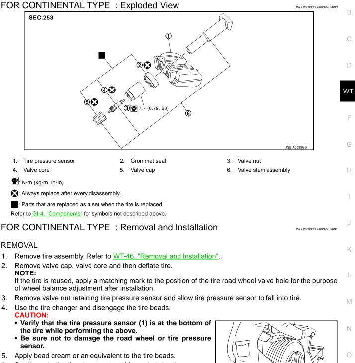
6. Set tire onto the tire changer turntable so that the tire pressure sensor inside the tire is located close to the road wheel valve hole.
