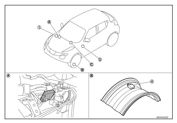
ABS actuator and electric unit (control 2. unit) Refer to <u>BRC-9, "Component Parts</u> <u>Location"</u>. BCM Refer to <u>BCS-6, "BODY CONTROL</u> <u>SYSTEM : Component Parts Loca-</u> <u>tion"</u> (With intelligent key system), <u>BCS-93, "BODY CONTROL SYS-</u> <u>TEM : Component Parts Location"</u> (Without intelligent key system).
