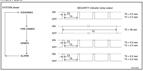
BCM shifts the phase as follows and the phase information is sent to siren control unit via communication line.
