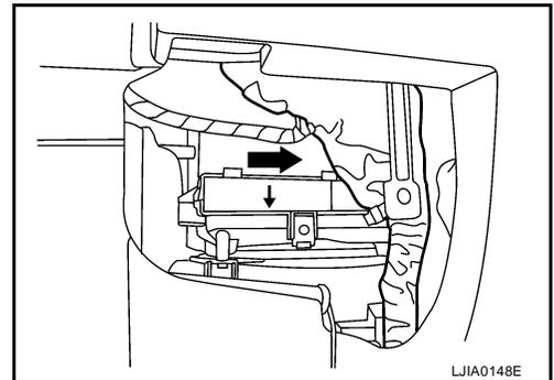
5. Install the in-cabin microfilter cover.
