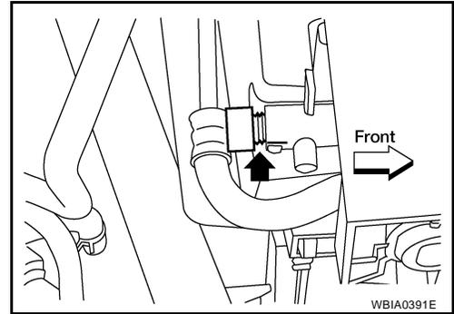
4. When draining all of the coolant in the system for engine removal or repair, it is necessary to drain the cylinder block. Remove the RH cylinder block drain plug to drain the right bank and the oil cooler hose to drain the left bank as shown.
