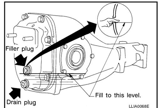
3. Install the filler plug and tighten to specification.
