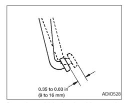
Press the pedal by hand and be sure the free travel is within the limits shown above. If free travel is out of the range shown above, see an authorized NISSAN dealer.
