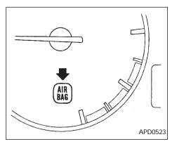
The supplemental air bag warning light, displaying BAG in the instrument panel, monitors the circuits of the supplemental air bag system. The circuits monitored by the supplemental air bag warning light are the diagnosis sensor unit, supplemental air bag modules and all related wiring.
