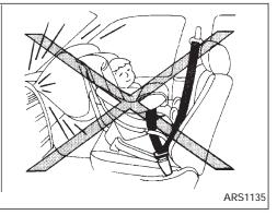
Failure to use the retractor's locking mode will result in the child restraint not being properly secured. The seat could tip over or otherwise be unsecured and cause injury to the child in a sudden stop or collision.
