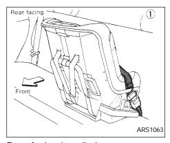
Rear facing installation on rear seat Center lap belt
