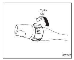
To turn the front fog lights on, rotate the switch to the (1) position.
