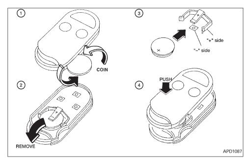
Replace the battery in the multi-remote controller as follows:
