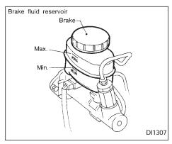
Check the brake fluid level in the reservoir. If the fluid level is below the MIN line or the brake warning light comes on, add **DOT 3** fluid up to the MAX line. If fluid must be added frequently, the system should be thoroughly checked by an authorized NISSAN dealer.
