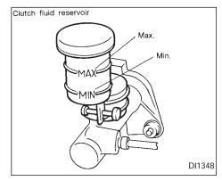
Check the clutch fluid level in the reservoir (manual transmission only). If the fluid level is below the MIN line, add **DOT 3** fluid up to the MAX line. If fluid must be added frequently, the system should be thoroughly checked by an authorized NISSAN dealer.
