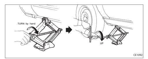
point. Align the jack head between the two notches in the front or the rear as shown. Also fit the groove of the jack head between the notches as shown
