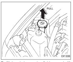
To fill the window washer fluid reservoir, lift the cap off the reservoir tank and pour the window washer fluid into the tank opening.
