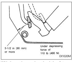
With the engine running, check the distance between the upper surface of the pedal and the metal floor. If it is out of the range shown above, see an authorized NISSAN dealer.
