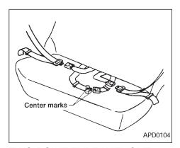
TWO-POINT TYPE WITHOUT RETRACTOR (rear center lap belt)
