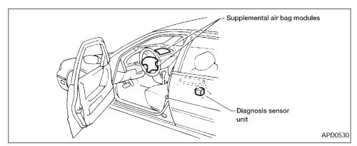
The driver supplemental air bag is located in the center of the steering wheel. The front passenger supplemental air bag is mounted in the dashboard above the glove box.
