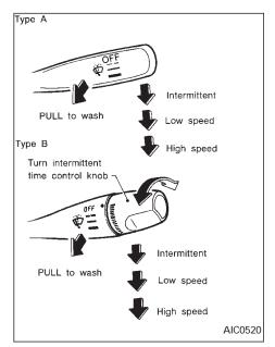
Push the lever down to operate the windshield wipers. Pull the lever toward you to operate the washer.
