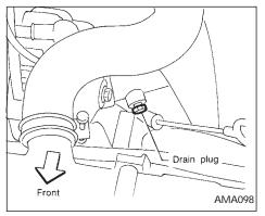
11. Check the radiator drain plug and the drain plug on the engine water pipe for any sign of leakage, tighten if necessary.
